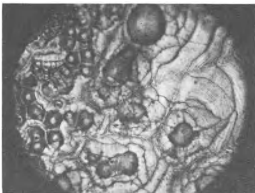
Fig. 46. Coalescence of primary and secondary oxides in 1% sulfuric acid with 45 V at \pm 1^\circ\text{C} after 100 sec ( 250\times ). (Reproduced at 65%.)
