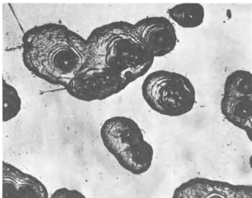
Fig. 12. Formation of primary oxide nuclei and secondary zone of oxidation after 15 sec in 1–5% sulfuric acid with 30–40 V at \pm 1^\circ\text{C} ( 200\times ). (Reproduced at 70%.)
