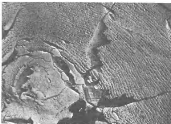
Fig. 38. Concentric arrangement of pores around the primary oxide nucleus in an oxide layer prepared in 1 % sulfuric acid with 35 V at \pm 1^\circ\text{C} . Electron micrograph ( 10,000\times ). (Reproduced at 65 %.)
