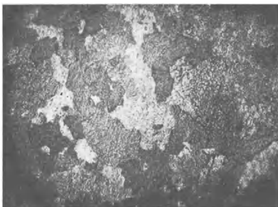
Fig. 67. Oxide coating after 15 min on variously oriented surfaces of chemically etched 99.99Al in 1% sulfuric acid at 40\text{--}45\text{ V} at \pm 1^\circ\text{C} , in polarized light ( 250\times ). (Reproduced at 65%.)
