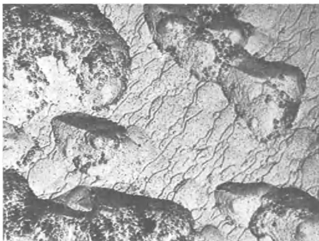
Fig. 28. Formation of oxide agglomerations at the surface of active subgrains during the first few seconds of anodic oxidation in 1 % sulfuric acid at \pm 1^\circ\text{C} with 50 V. Electron micrograph ( 20,000\times ). (Reproduced at 80 %.)
