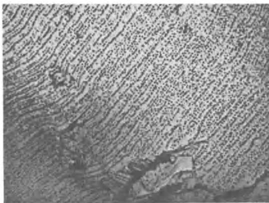
Fig. 39. Rows of pores along the reaction waves of the secondary zones of oxidation in an oxide layer prepared in 1% sulfuric acid at 35 V. Electron micrograph ( 10,000\times ). (Reproduced at 65%.)
