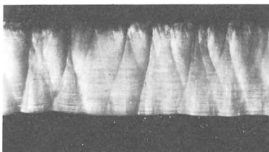
Fig. 43. Micrograph of the heavy hard oxide layer prepared in 1% sulfuric acid at 50 V, in polarized light. ( 150\times ). (Reproduced at 65%.)
