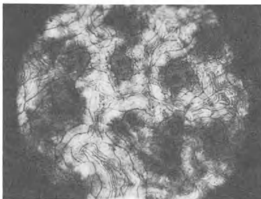
Fig. 47. Same as Fig. 46. Gradual coalescence of primary and secondary oxides formation period of the covering oxide layer after 5 min ( 250\times ). (Reproduced at 65%.)
