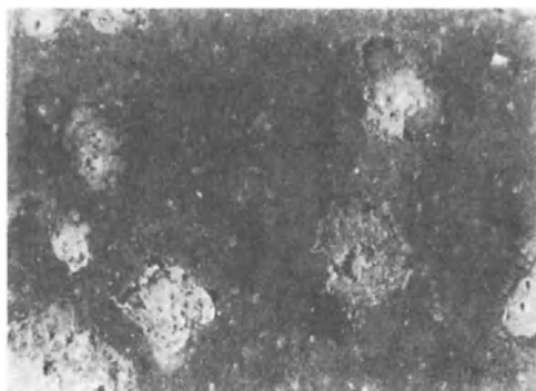
Fig. 87. Destruction of layer by pitting ( 50\times ). (Reproduced at 65%.)
